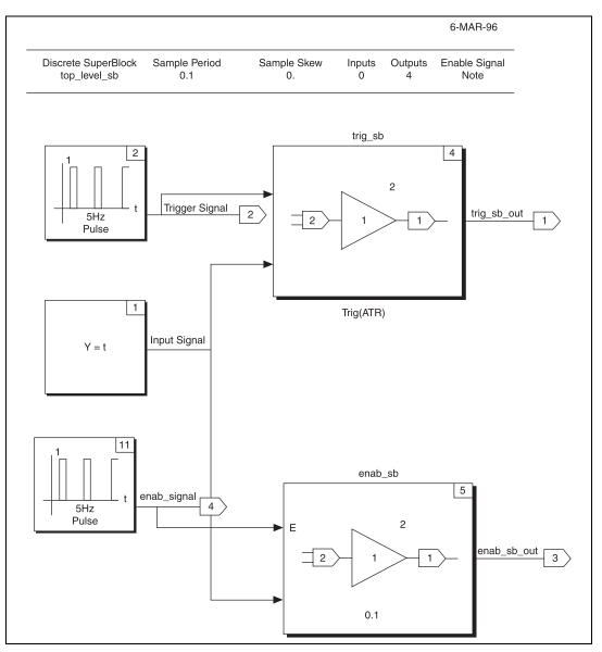
Figure 8-1. Model with Enabled and Triggered Tasks
